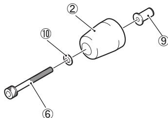
6. Install the Front Axle Slider (L) ② to the motorcycle.
